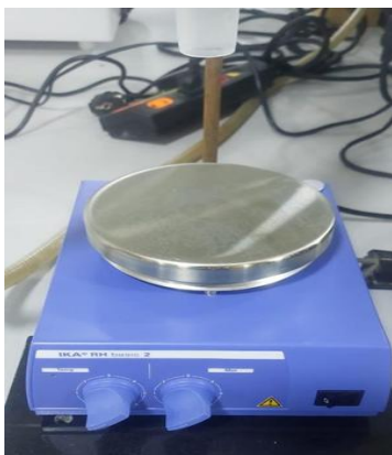
Figure 2. Magnetic stirrer device (IKA RH basic 2 model).
